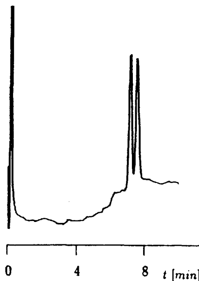
Fig. 6. Enantiomer separation of o,p' -DDT standard solution on a 10 m capillary column (0.25 mm ID) coated with heptakis(2,6-di-O-methyl-3-O-trifluoroacetyl)- \beta -cyclodextrin bonded to dimethylpolysiloxane (Chirasil-Dex-TFA) [4].
